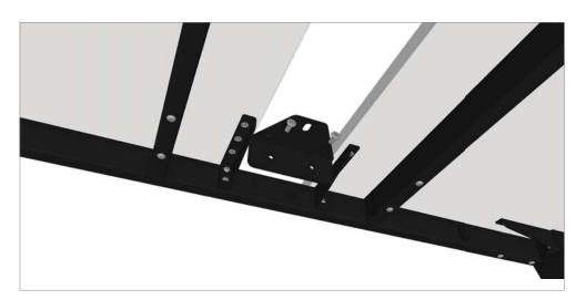
**STEP 1:** Fix AXSB bracket to end frame and tighten.
